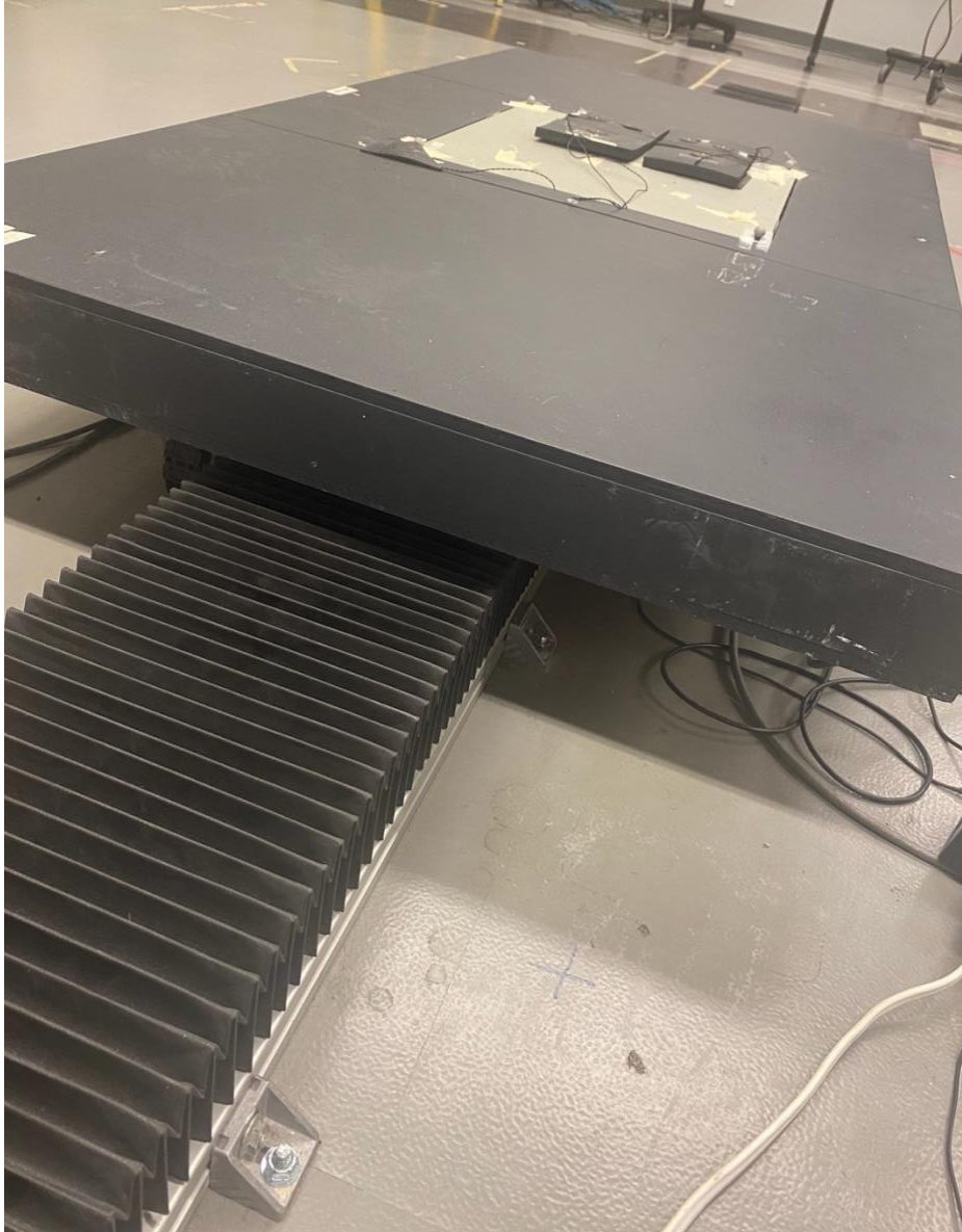
Figure 1: The surface translation platform used in this experiment. Note the force plate that was embedded in the middle of the wooden surround and the rubber pads, containing the vibrating factors, were placed on top of the force plate.
