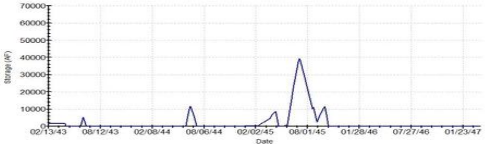
Figure 7: Water bank storage under multi-year drought conditions (2043-2046) Scenario: 3yr Min (CGCM 3T47 3B1), 30-year record
