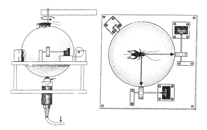
sphere, at 90° intervals, are four speakers (Linear, B-4-5 JO full-range frequency) through which songs are broadcast. Each speaker is 35.4 cm from the centre of the top of the sphere.
